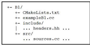
Here, exampleB1.cc contains main() for the application, with include/ and src/ containing the implementation class headers and sources respectively.
