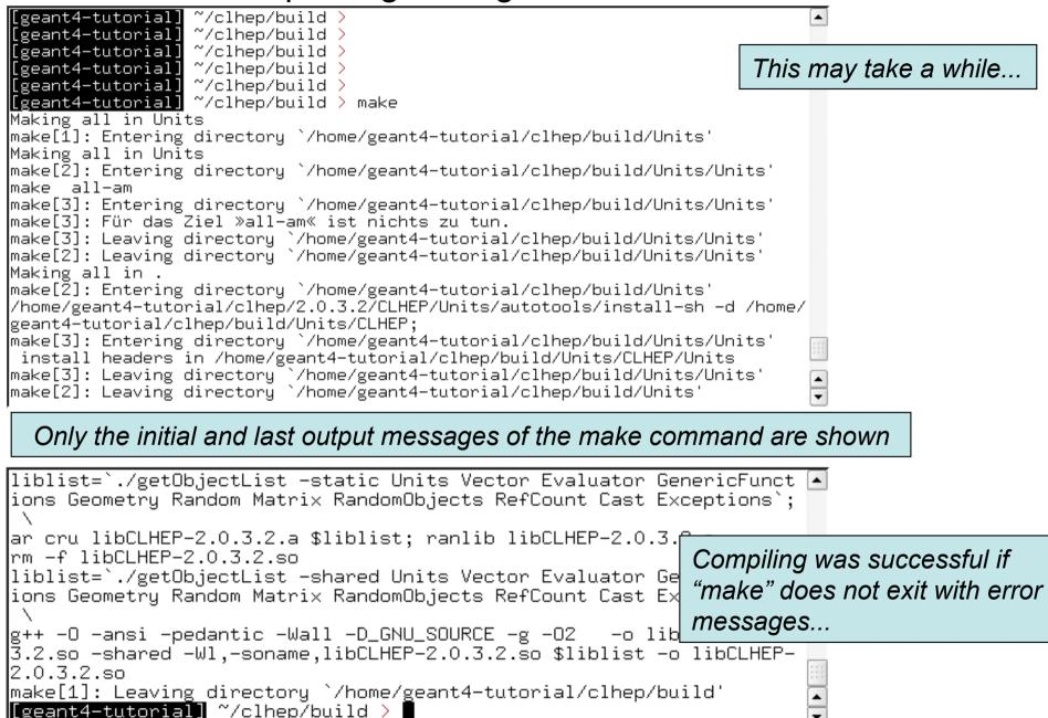
Once the package was compiled successfully, CLHEP can be installed using the "make install" command:
