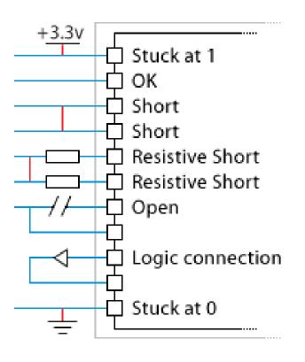
Chip manufacturers includes special cell on each of the ICs pins to facilitate test.
