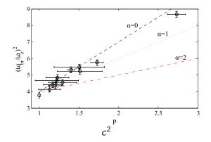
Experimental frequency ratio  $(\omega/\omega_0)^2$  vs compression factor  $c^2$ Theory = dashed line. From top to bottom, force exponent  $\alpha = 0, 1, 2$ .
