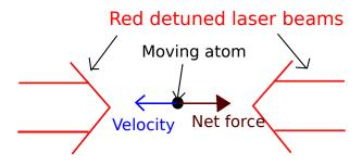
Doppler effect  $\rightarrow$  a friction Spatial trapping: through a magnetic field gradient, or a dipolar trap.
