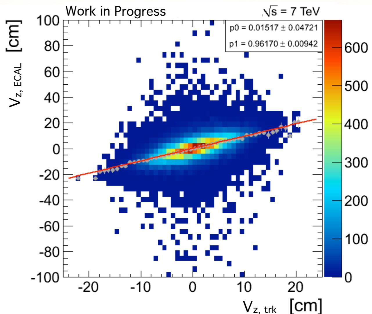
**Linearity 1:1** between  $V_{z,\text{ECAL}}$  and  $V_{z,\text{trk}}$
