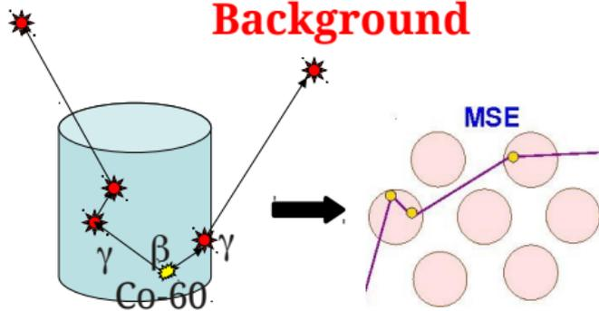
Point-like (single-site) energy deposition inside one HP-Ge diode (Range:  $\sim 1\text{mm}$ )
