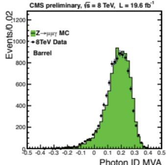
Good agreement data/MC for cut-based ( $Z \rightarrow ee$ ) and MVA ( $Z \rightarrow ee\gamma$ )
