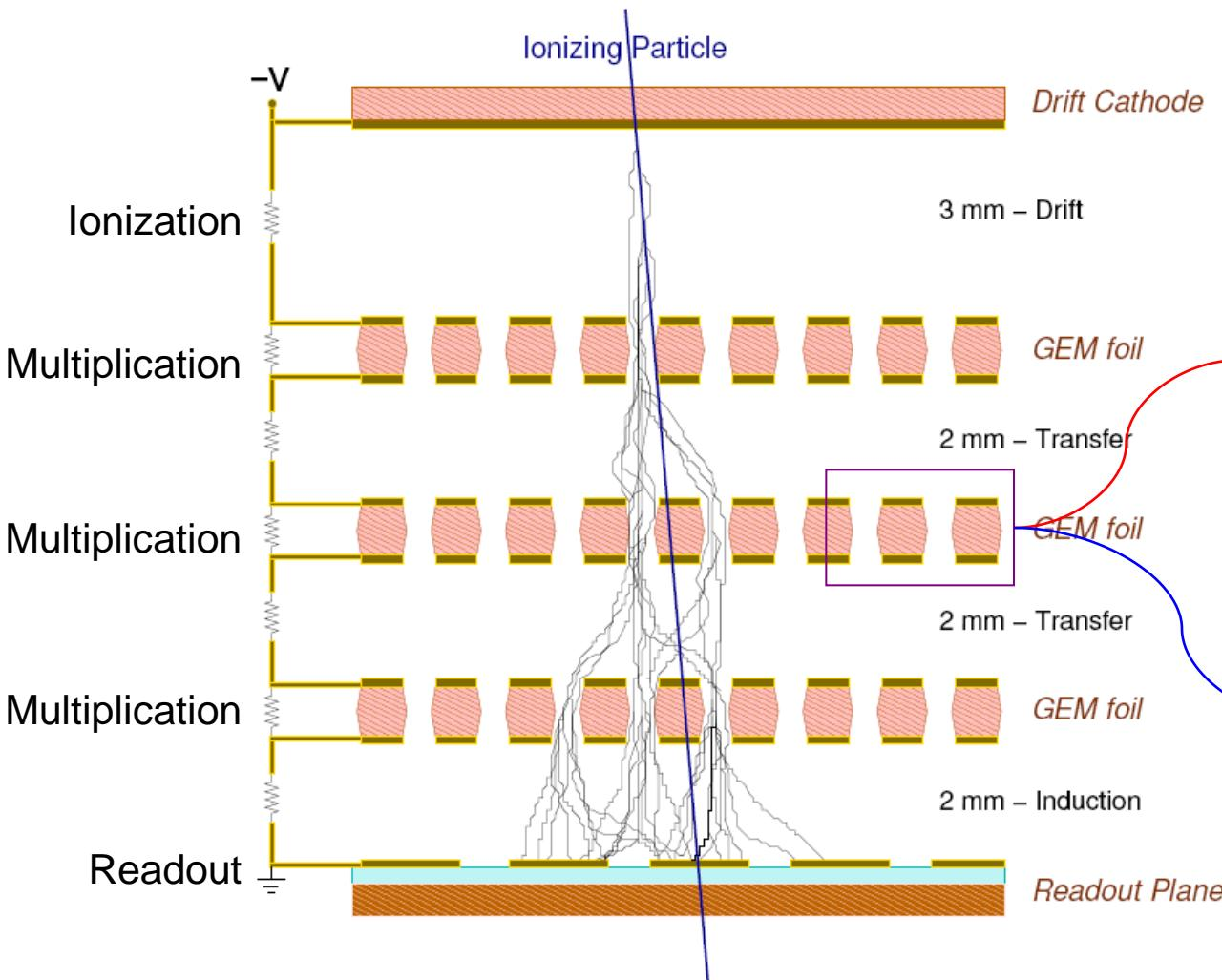
GEM foil: 50  $\mu\text{m}$  Kapton + few  $\mu\text{m}$  copper on both sides with 70  $\mu\text{m}$  holes, 140  $\mu\text{m}$  pitch
