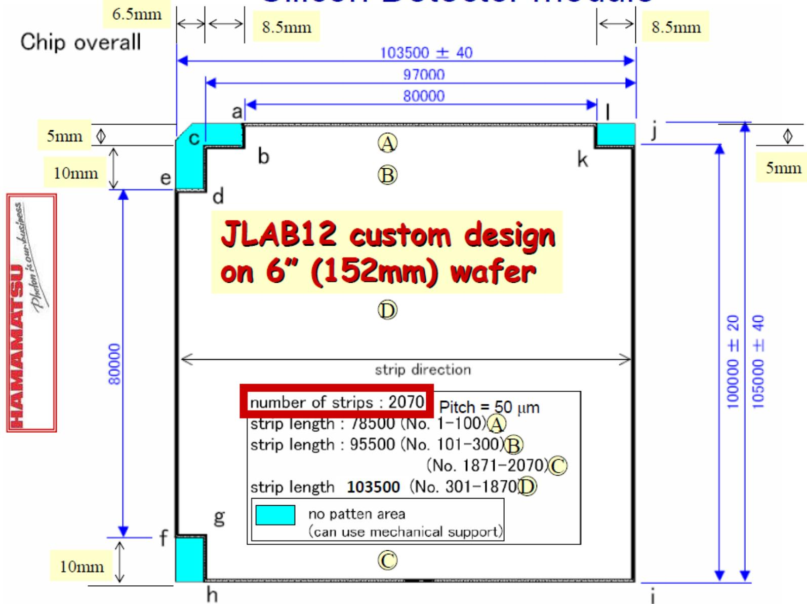
μSiD composed by 2 planes (x/y) each made of 2 of the above modules
