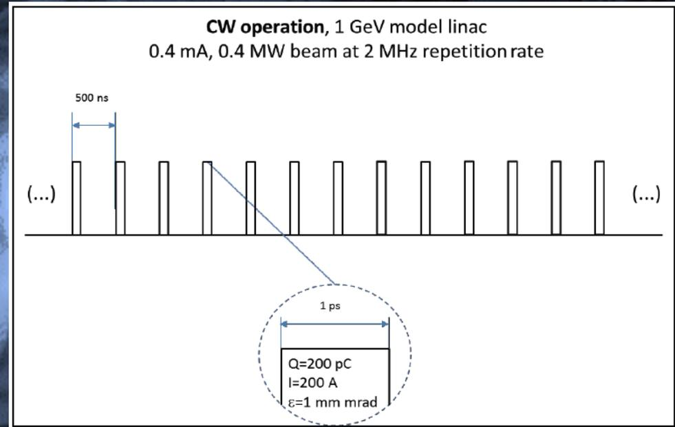
The **CW** or **qCW** choice, combined with a proper bunch distribution scheme, offers the **most versatile solution to provide bunches to a number of different experiments**, as could be envisaged in a multi-purpose facility.
