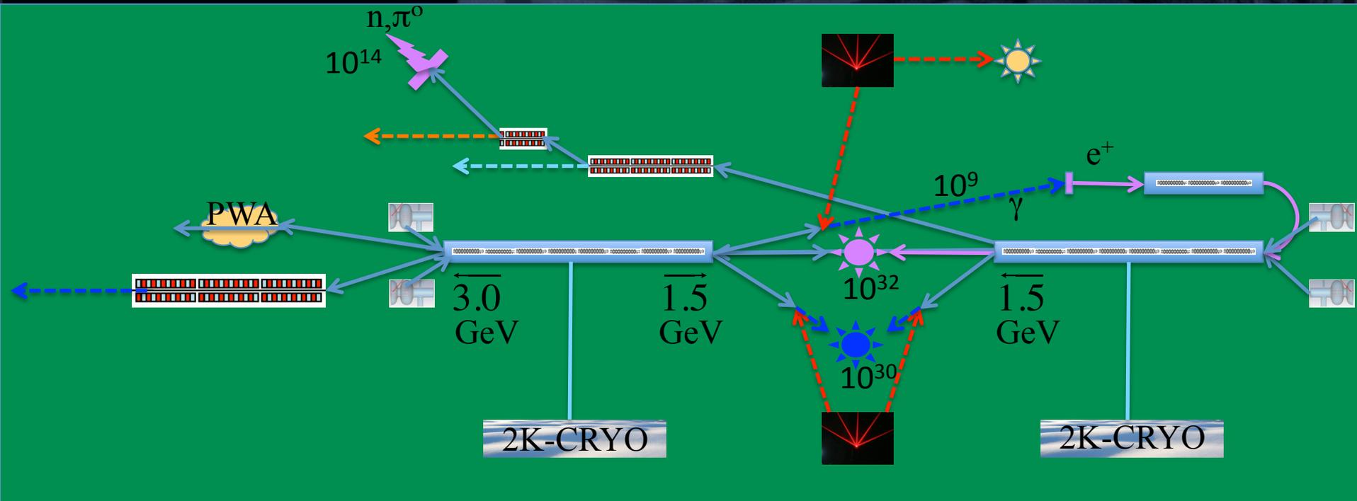
Based on a combination of a **high duty cycle radio-frequency superconducting electron linac** (SC RF LINAC) and of **high energy lasers** it will be able to produce a high flux of **electrons, photons (from infrared to  $\gamma$ -rays)**, neutrons, protons and eventually **positrons**, that will be available for a wide national and international scientific community interested to take profit of the most advanced particle and radiation sources.
