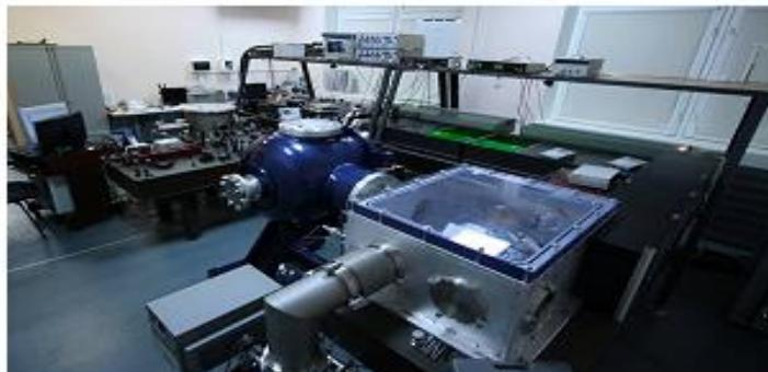
**Subterawatt femtosecond Ti:Sapphire kilohertz laser system**
