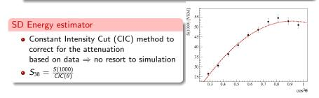
Calibration of the SD energy estimator: with hybrid events
