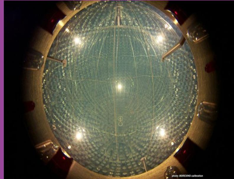
Figure 6: *The Borexino detector, located in the Gran Sasso laboratory (Italy). Its ultrapure scintillator permits us to observe the electrons-or positrons-which are occasionally hit by neutrinos-or antineutrinos, even when their energy is below MeV.*
