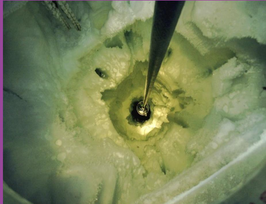
Figure 7: *The IceCUBE detector (South Pole). It reveals the (anti) muons occasionally produced by (anti) neutrinos. It can get some information on supernova ( $\sim 10$  MeV)  $\bar{\nu}_e$ 's thanks to its huge mass but it is optimized for high energy ( $> \text{TeV}$ ) neutrinos.*
