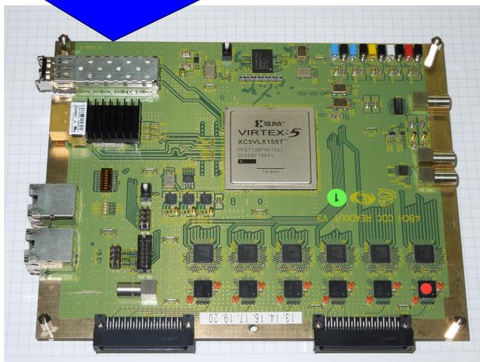
prototype of readout board
