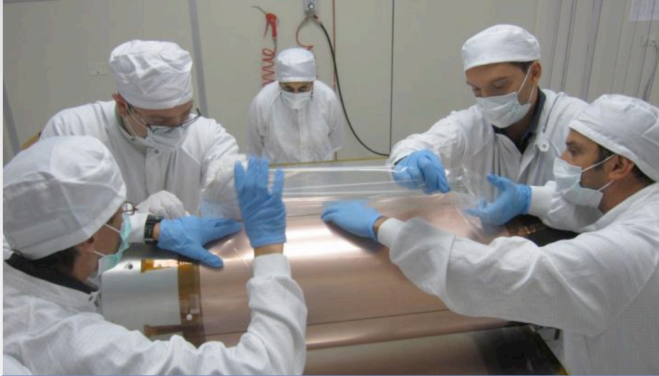
GEM is protected with a Mylar sheet and wrapped on the cylindrical mold
