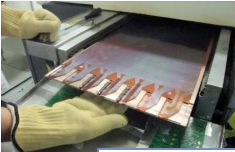
Circuit are put in the reflow oven with monitored temperature cycle , for connectors soldering
