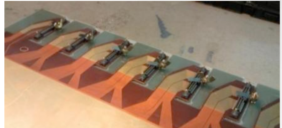
Connectors are placed and fixed on the circuit after the deposition of the solder paste with a serigraphy machine
