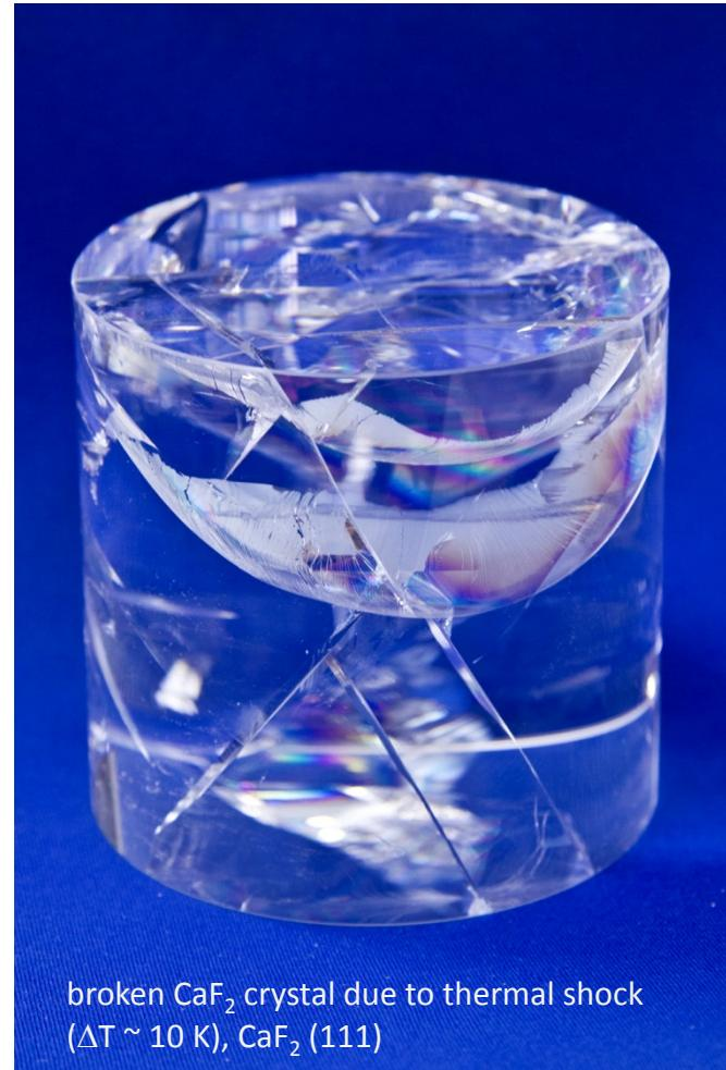
broken CaF<sub>2</sub> crystal due to thermal shock
