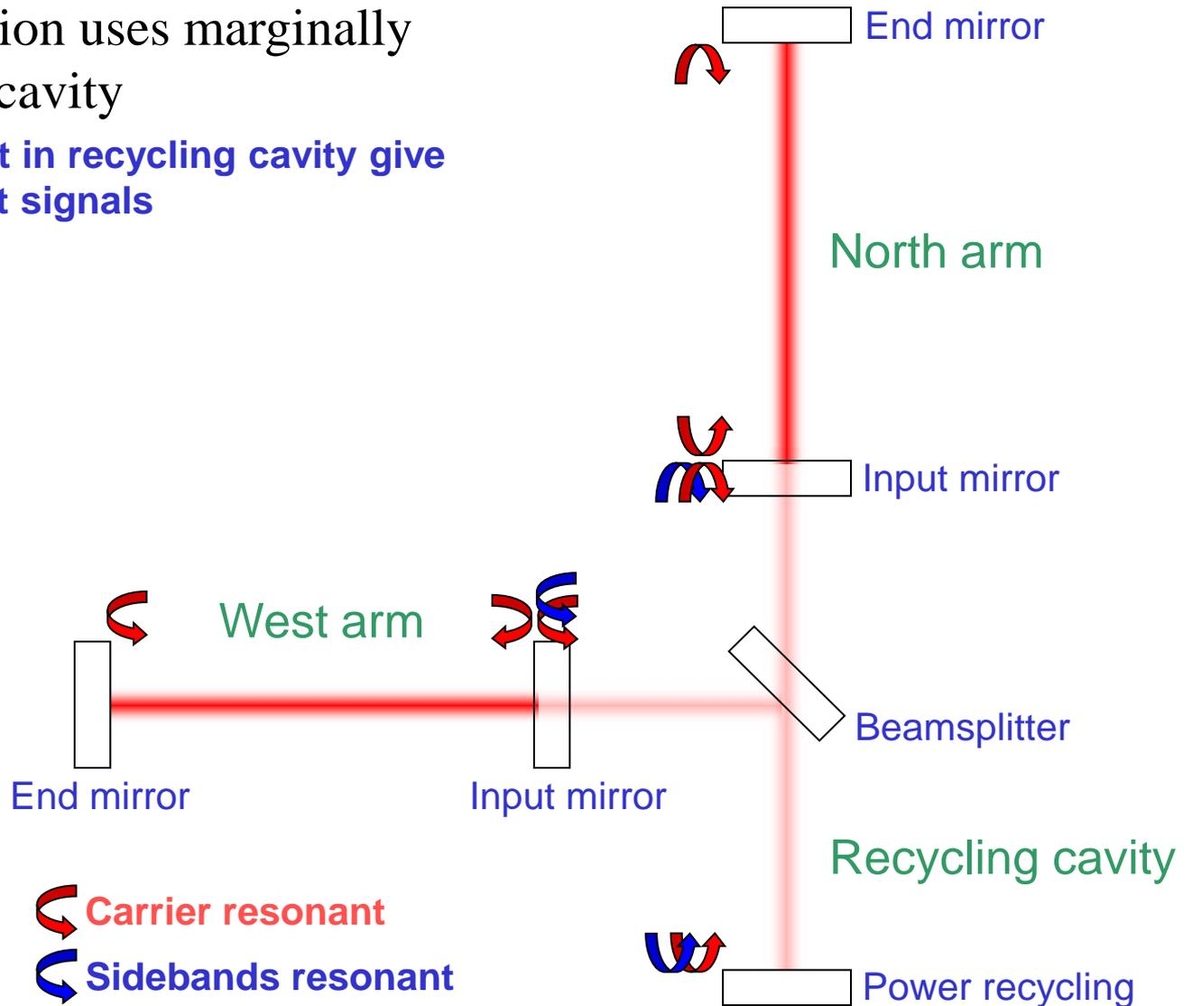
Virgo configuration uses marginally stable recycling cavity
