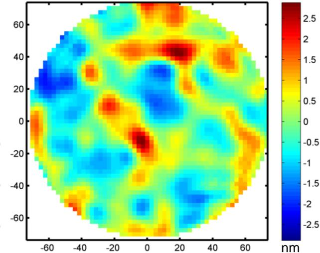
Frequency independent reconstruction looks washed out due to attenuation of high frequencies
