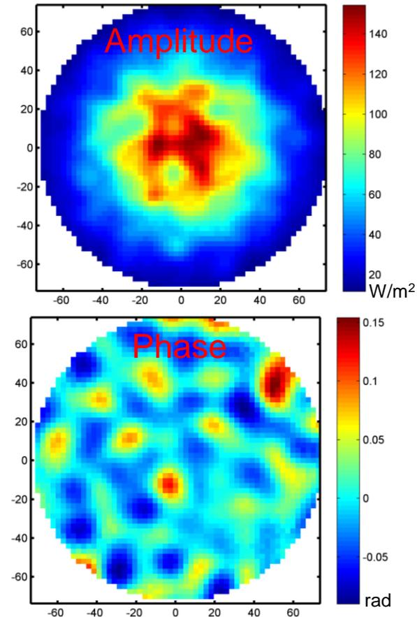
Recycling gain of TEM00 increases from 23% to 99.4% in 40 iterations
