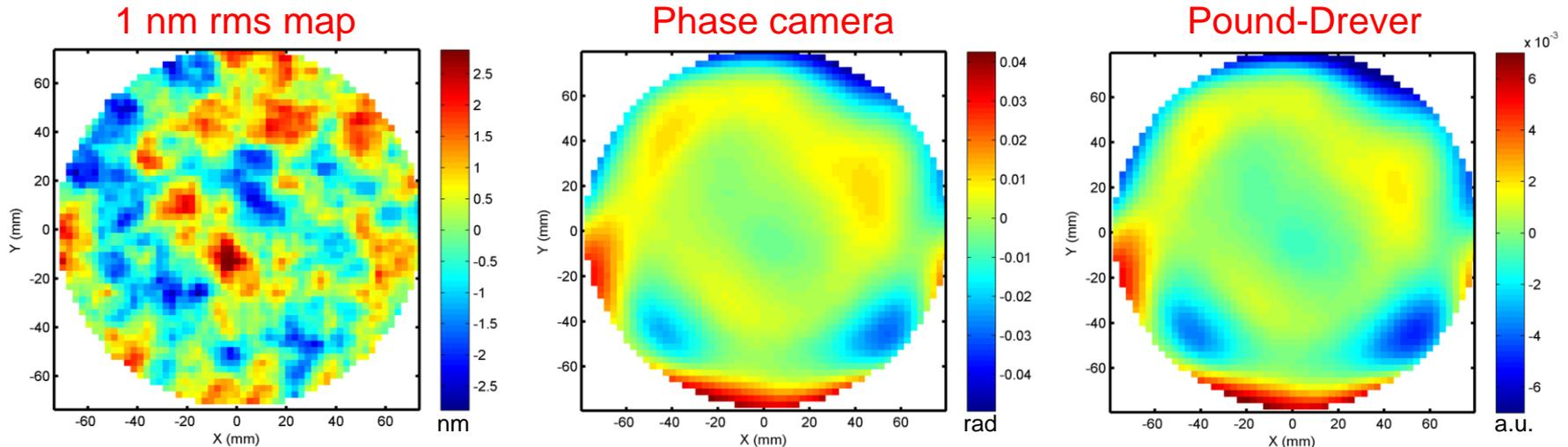
Results are less clear due to large round-trip Gouy phase in recycling cavity
