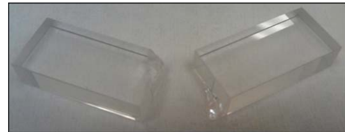
Sapphire bonded samples which broke across the bond surface, but with damage to the bulk sapphire. Strengths 60-80MPa at 77K
