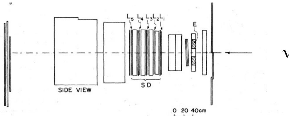
FIG. 1. Diagram illustrating the experimental arrangement; V, veto counter; C<sub>0</sub>, NG spark chamber; E, six emulsion stacks on frame; S<sub>0</sub>, scintillation counter; WG, wide-gap spark chamber; SD, shower detector comprising scintillator counters S<sub>1-4</sub>, NG spark chambers C<sub>1-4</sub> and lead plates L<sub>1-5</sub>; M, muon identifier.
