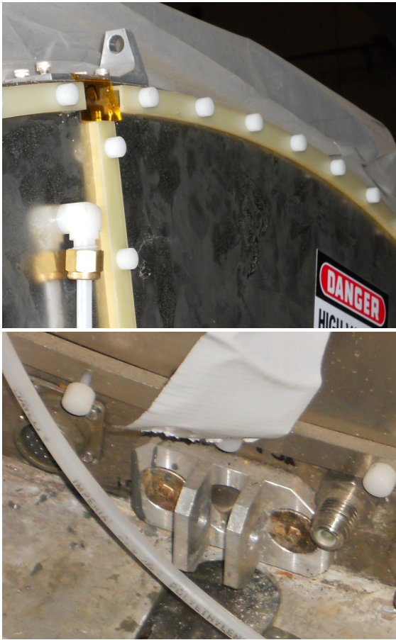
Figure 7.22: Forward end mounting system on the BABAR drift chamber. (a) Tab on the outer radius of the drift chamber. (b) Corresponding mounting point on the CST.
