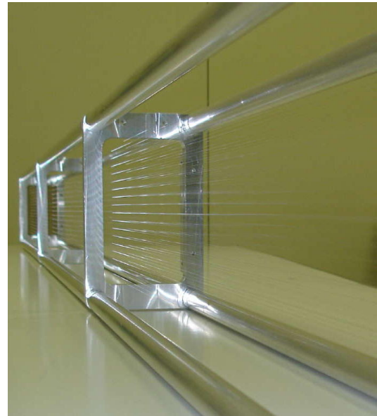
Figure 7.6: Prototype 2: detail of the strung wires.
