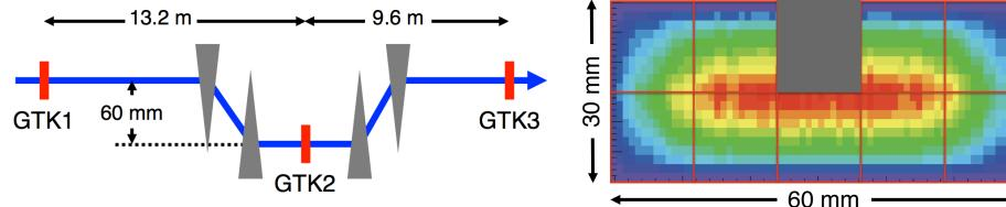
Pixel size 300 × 300  $\mu$ m<sup>2</sup> →  $\sigma_p/p$  ~ 0.2%,  $\sigma_{\theta}$  = 16  $\mu$ rad
