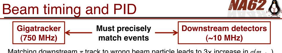
Matching downstream  $\pi$  track to wrong beam particle leads to 3× increase in  $\sigma(m_{miss})$ Use detectors with good time resolution to avoid mismatching:
