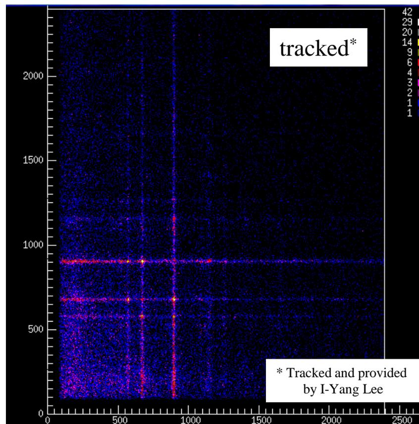
Reduction of Compton background by tracking allows – for the first time – gamma spectroscopy with fast beams with spectral quality comparable to arrays with anti-Compton shield, i.e. GammaSphere.
