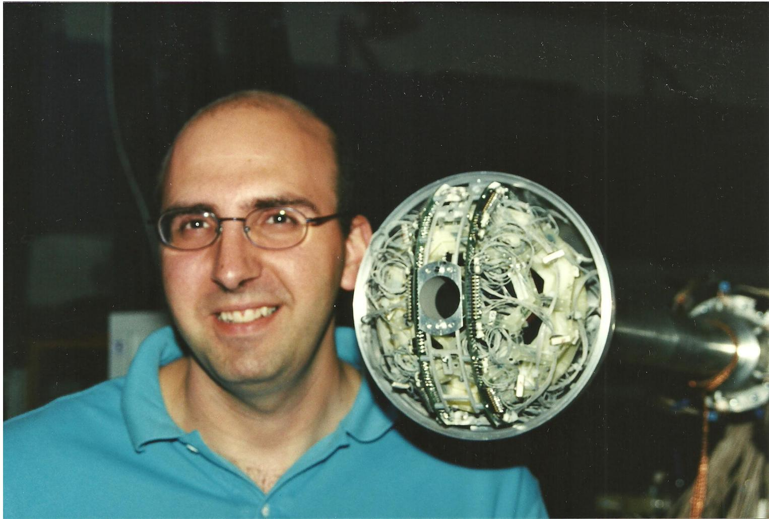
40  $\Delta E$  (130 $\mu m$ , mounted in reverse configuration)+E(1mm) telescopes
