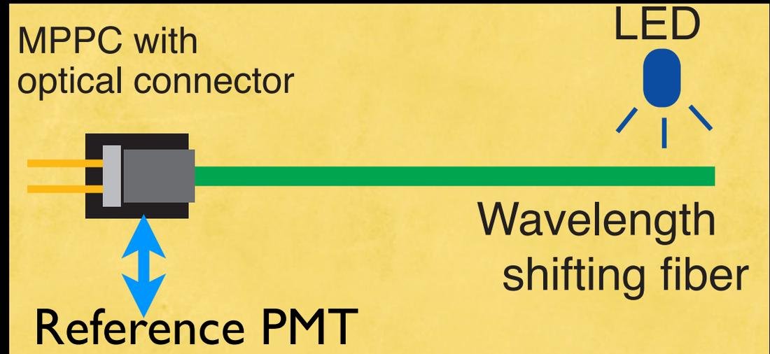
Optical connector developed to ensure good contact.
