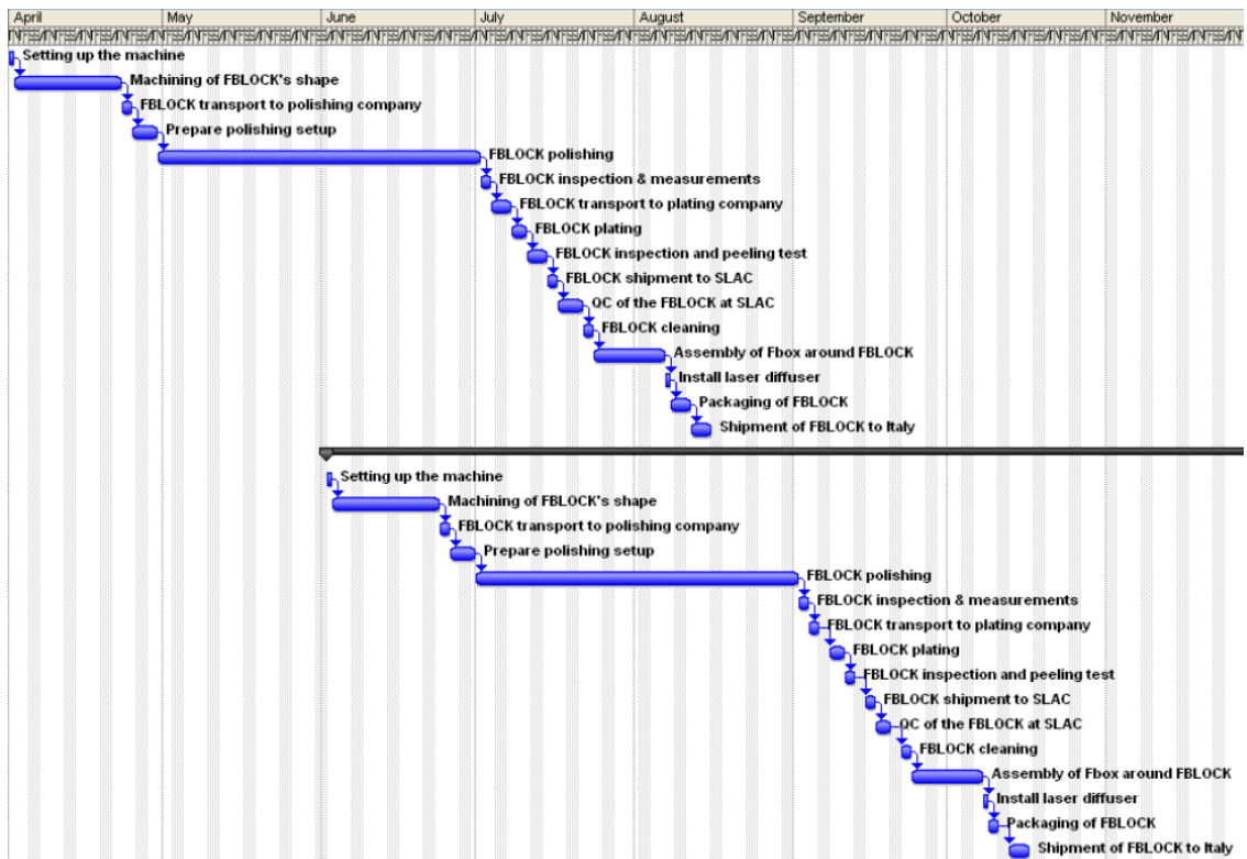
Figure 8.68: FBLOCK production schedule (2 FBLOCK production cycles only).
