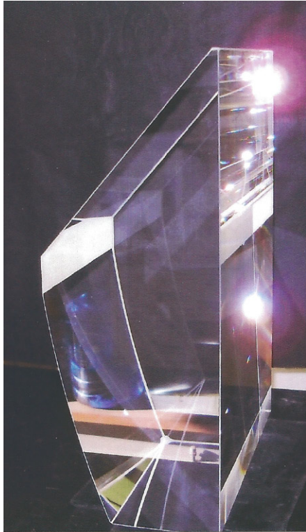
(a) FBLOCK after polishing but before plating.
