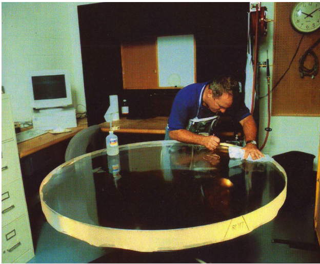
Figure 8.38: An example of the fused silica 7980 material in the form of a 60 inch dia. boule made by Corning.
