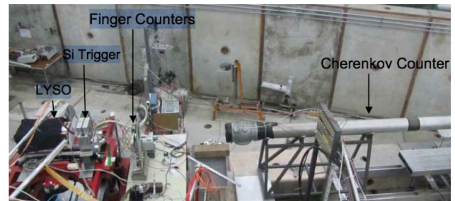
Figure 9.29: Schematic view of the test beam setup used at CERN.
