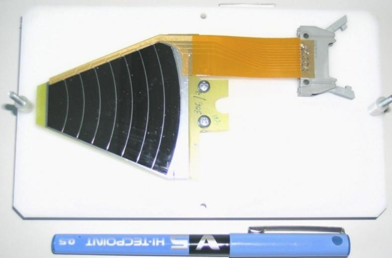
When the detector is mounted at 5 cm distance from the target the coverage of the polar angle  $\theta$  is about 42 degrees (from 18 to 60 degrees)
