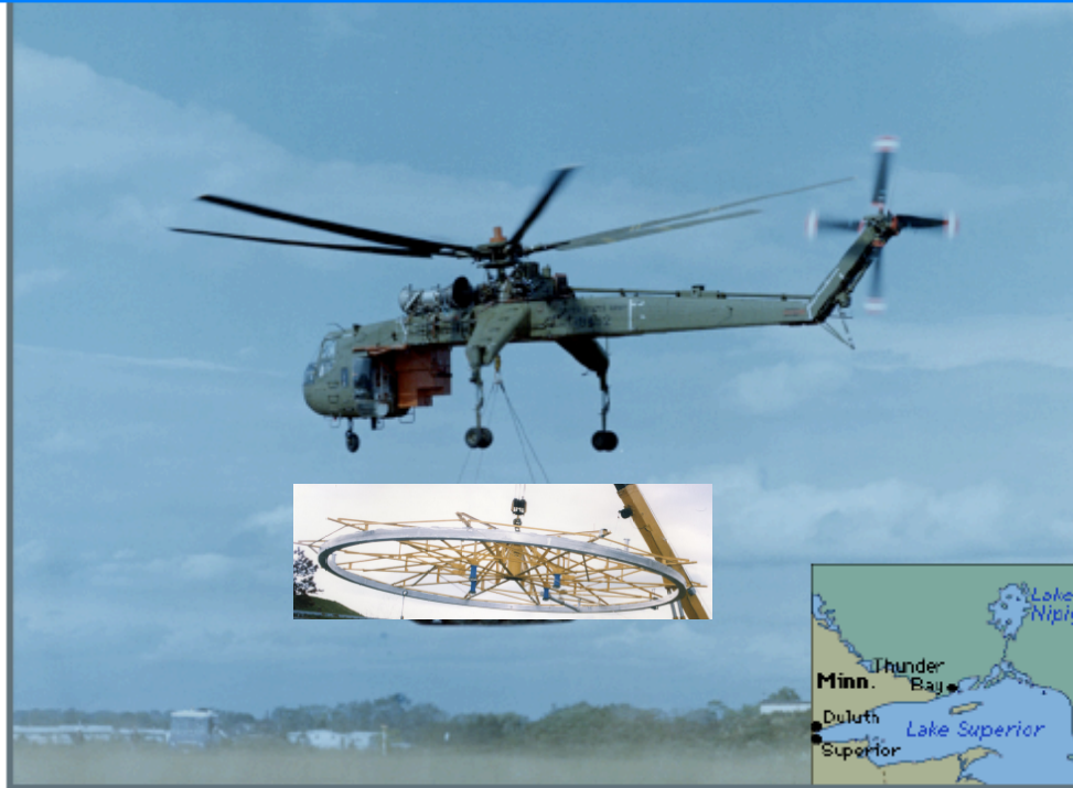
Sikorsky S64F 12.5 T hook weight (Outer coil 8T)
