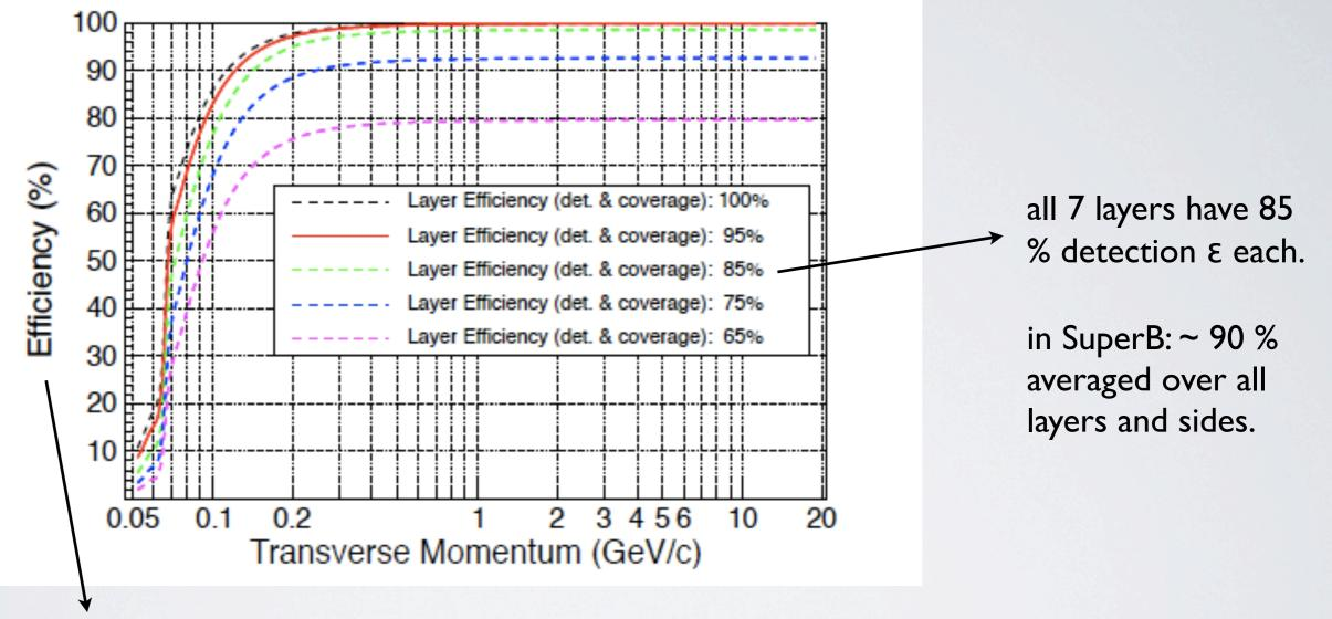
global tracking efficiency = detector efficiency x matching efficiency
