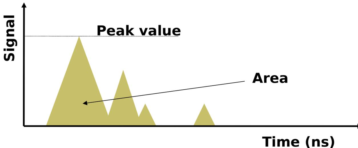
$$\text{AoP} = \text{Signal integral over Peak value}$$
