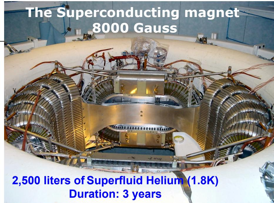
Expected life time of the AMS Cryostat on ISS:
