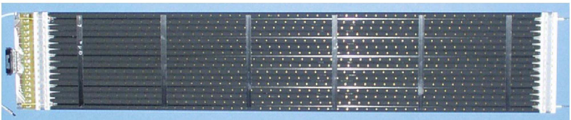
5,248 tubes selected from 9,000, 2 m length centered to 100µm, verified by CAT scanner
