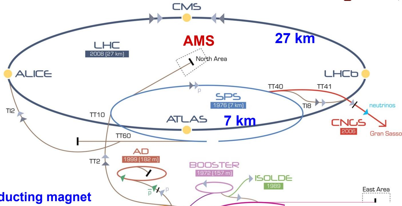
with superconducting magnet
