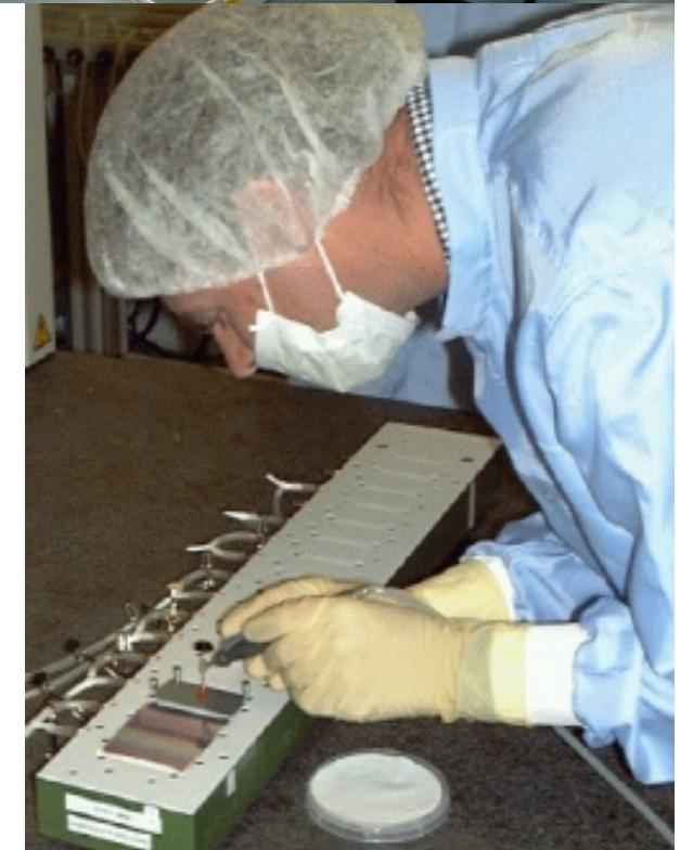
**There are 9 planes with 200,000 channels aligned to 3 microns**
