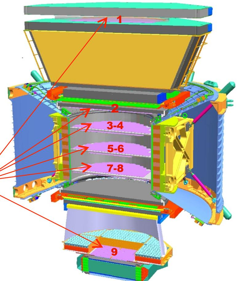
Layers 1 and 9 are far away from the magnet to extend the lever arm.
