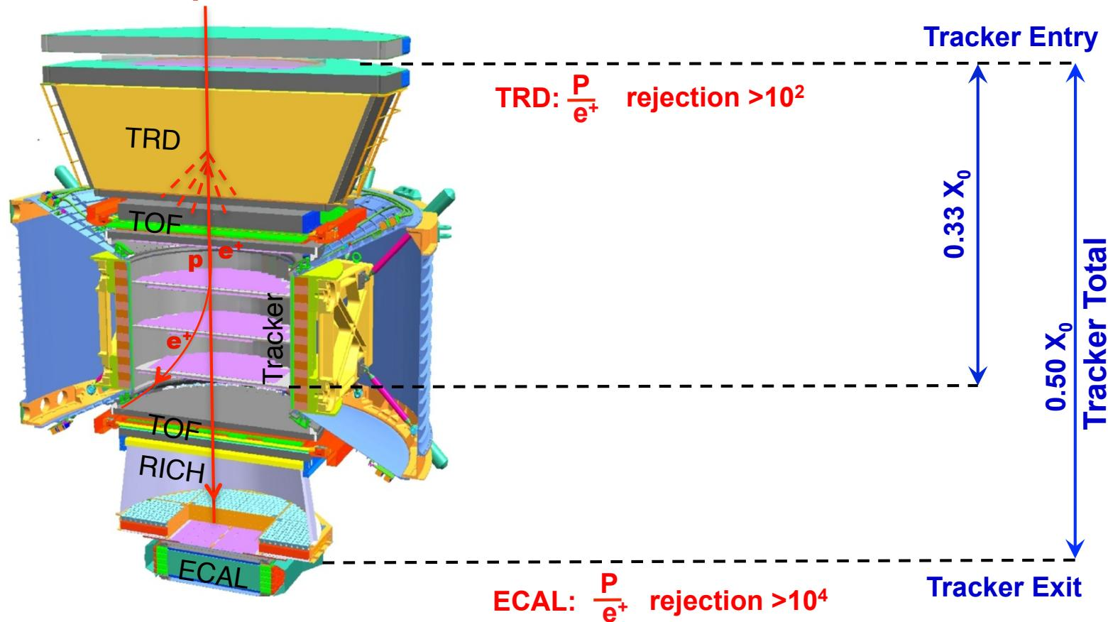
a) Minimal material in the TRD and TOF
