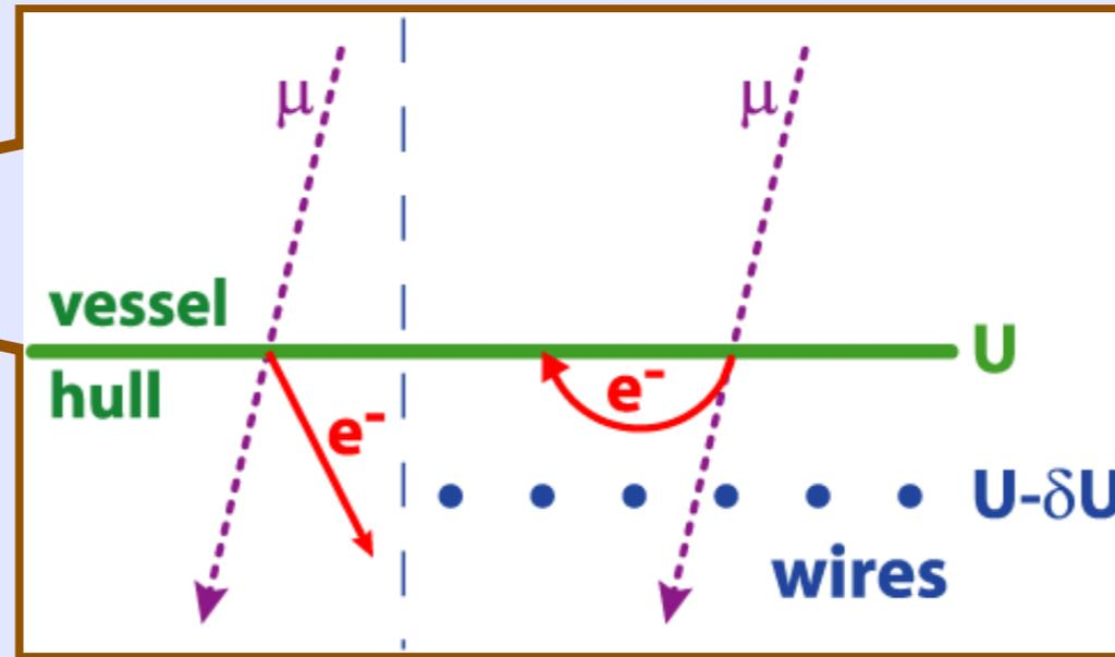
Cosmic rays knock electrons from the vessel hull
