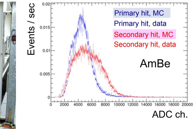
Regular AmBe source calibrations were used to monitor behavior of the detector and to normalize a Monte-Carlo description of the detector response. For each event a number of secondary hits within the DAQ window (60  $\mu$ s), hit time and energy were recorded. Time distribution of secondary hits was compared to AmBe data.
