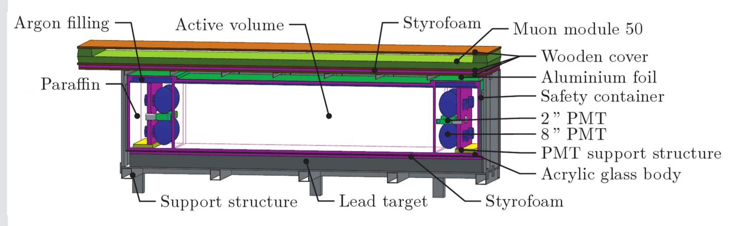
We have built and operated in 2009 - 2012 in Laboratoire Souterrain de Modane (LSM, 4800 mwe) a Neutron Counter (NC) detector based on 1 m<sup>3</sup> of Gd-loaded liquid scintillator viewed by 16 PMTs of 8-inch diameter. The system was coupled to a muon telescope to tag original muons. Underneath the detector there was 10-cm layer of Pb. The details can be found in Astropart. Phys. 34 (2010) 97.
