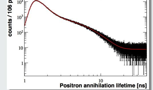
Fitted o-Ps time spectrum. All the fits give a normalized X<sup>2</sup> in the range [0.85 - 0.98].
