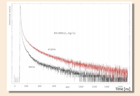
The light pulse from a scintillator is modeled as the superposition of three exponentials
