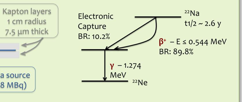
The <sup>22</sup>Na β<sup>+</sup> source is deposited between two identical Kapton layers. The source is placed in a vial containing the scintillator to be characterized, between two plastic scintillator detectors.
