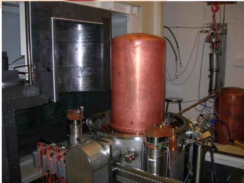
**400g “Interleaved Detectors”(ID) detectors.
