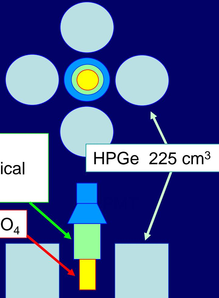
$^{106}\text{CdWO}_4$  in coincidence / anticoincidence with HPGe
