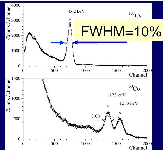
Excellent optical and scintillation properties thanks to special R&D to purify raw materials and Low-thermal-gradient Czochralski technique to grow the crystal
