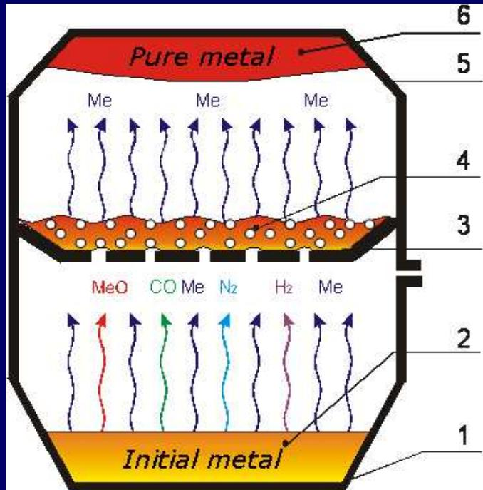
1 – crucible; 2 – initial metal; 3 – plate with holes; 4 – getter; 5 – condenser; 6 – purified metal
