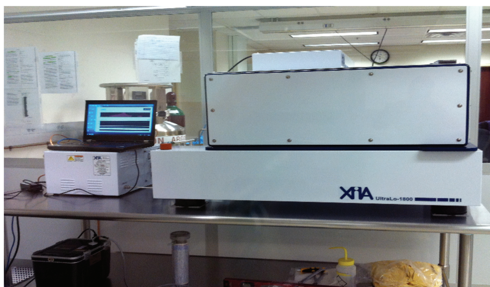
A low-background counting system: Peruna - XIA Alpha Particle Counter @SMU
