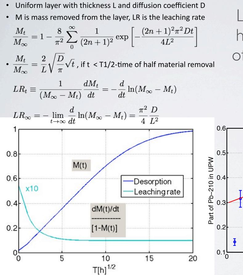
Leaching rate is defined here as the relative rate of material removal from the source.
