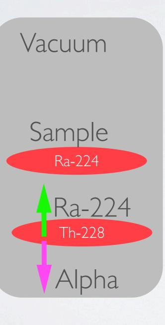
Thin source of Th-228 was prepared and put in vacuum chamber. The acrylic and stainless steel samples was placed above the source. Alpha-recoil Ra-224 was plated on the samples. The samples were alpha-counted before and after washing in various solvents: Water, LAB, Radiacwash, Nitric acid
