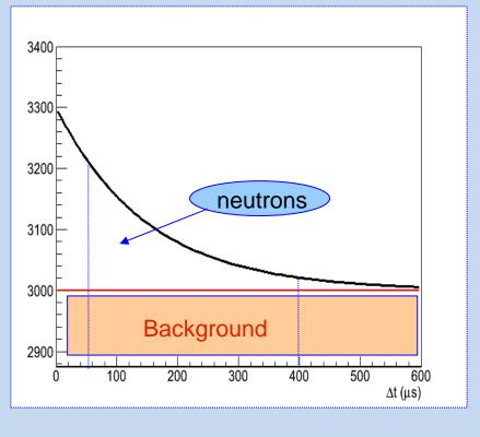
In LVD we can estimate the background component measuring the counting rate each time the gate in that counter is opened.
