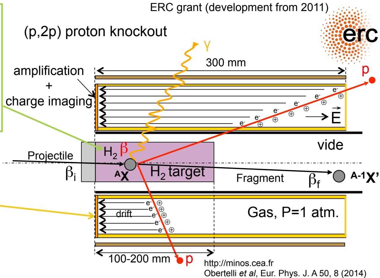
Initial goal: vertex resolution~4 mm FWHM, detection efficiency > 80%
