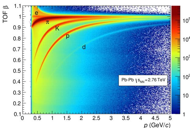
TOF: PID through particle velocity measurement
