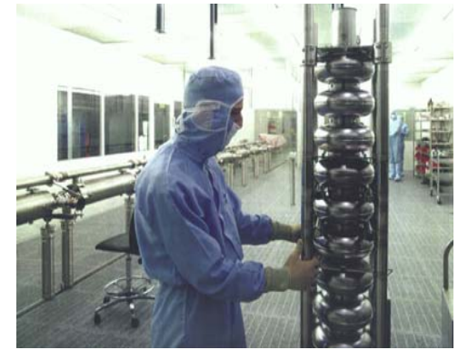
Cleanroom handling of niobium cavities
