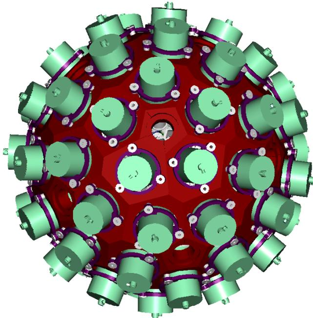
The innovative use of detectors in **position-sensitive mode** (combining **digital DAQ**, **PSA (Pulse Shape Analysis)**,  **$\gamma$ -ray tracking**) will result in high efficiency ( $\sim 40\%$ ), excellent energy resolution and **sensitivity** making AGATA the ideal device for spectroscopic studies of weak channels.
