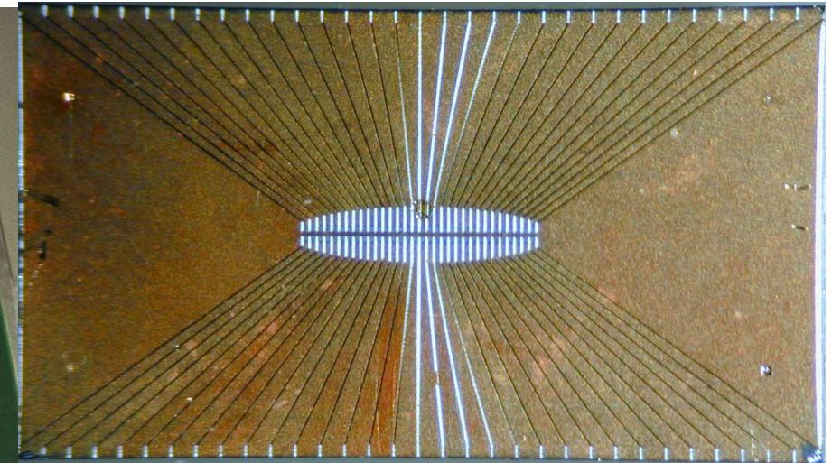
2D VIGO experimental semiconductor array detector (HgCdTe grown on a GaAs substrate - zoomed, up figure) and installed on a PCB with 60 dB amplifiers for each pixel signal (on the left)
