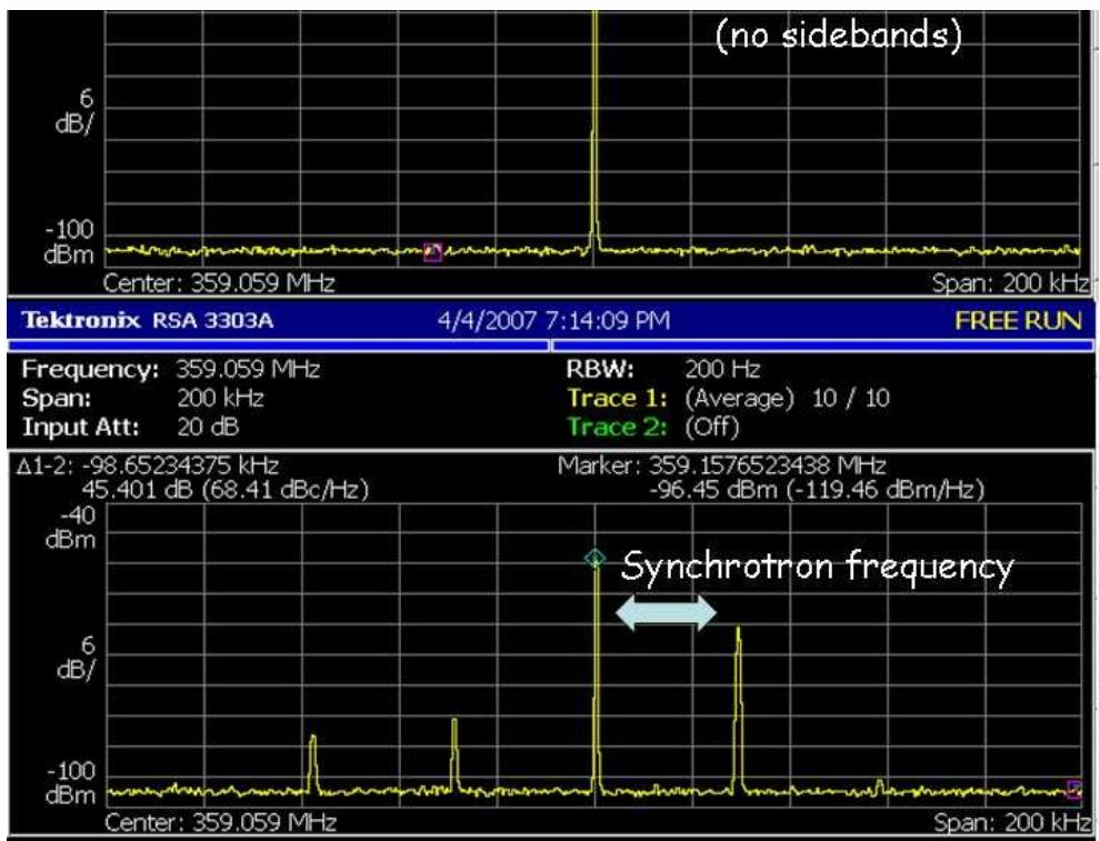
3+L beamline with single pixel detector and beam longitudinal behavior studies using LFB (left)
