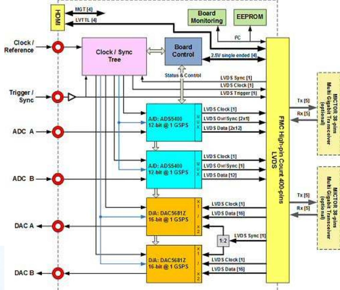
Coax connectors are SSMC, a type not currently used at LNF. So there is an extra-cost to interface them
