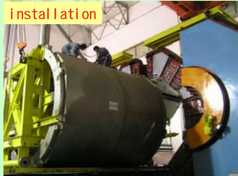
The magnet reached super-conducting status and 1T magnetic field at 3364A. Field mapping with SCQ completed Aug., 07
