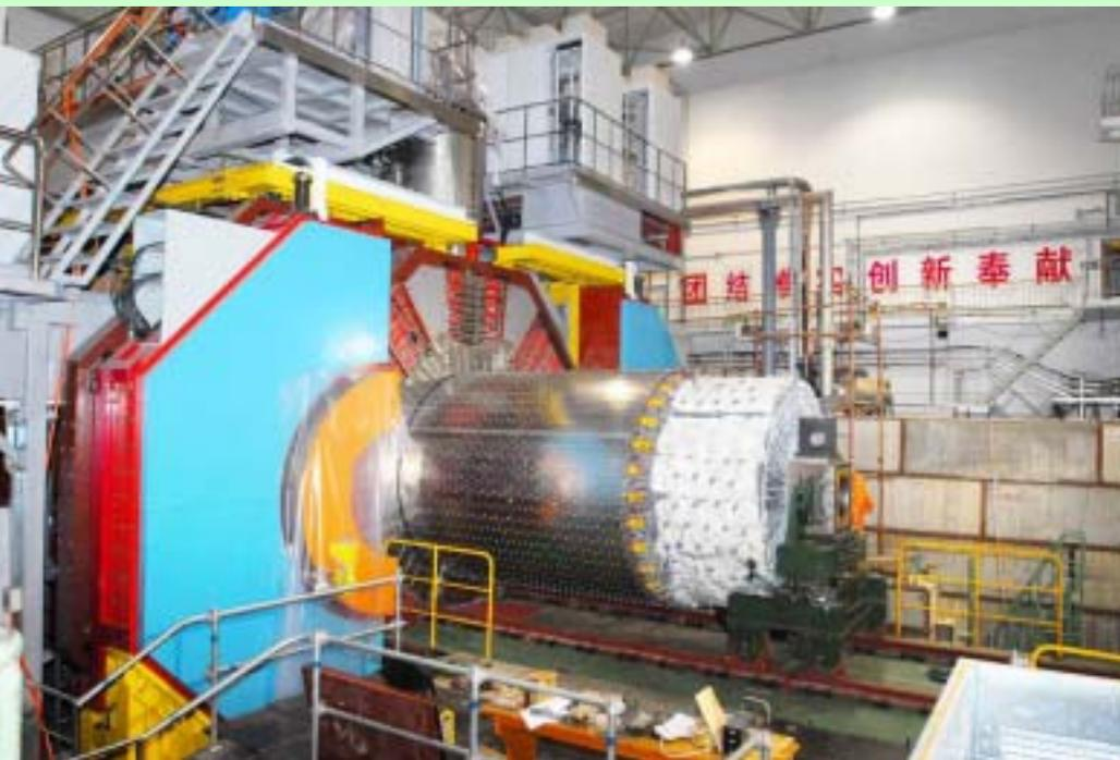
**Barrel EMC installed in the yoke**
