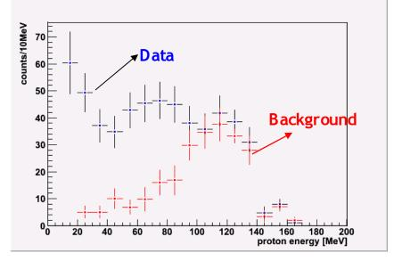
The background for the  $^5{}_{\Lambda}$ He has been evaluated by subtracting the proton spectrum in correspondence to the side-bins of the  $\pi^-$  spectrum (280-288 MeV/c)
