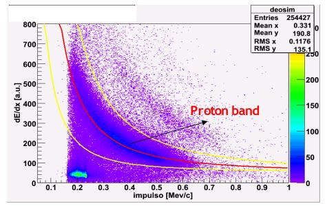
Proton selection asking the coincidence of protons identified with the two layers of drift chamber and the outer layer of silicon detector
