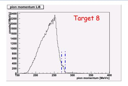
The top panels show the inclusive spectrum of negative pions for each <sup>6</sup>Li target and the bottom panel shows the sum of the two spectra.
