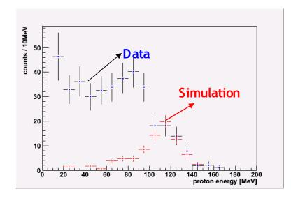
In the pion spectrum in coincidence with a proton the background corresponds to the reaction  $\begin{matrix} K^- & np & \longrightarrow \Sigma^- p \end{matrix}$  Followed by the decay  $\Sigma^- \longrightarrow n\pi^-$
