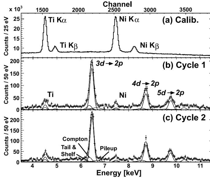
Figure 2: (a) A typical x-ray spectrum for self-triggered events which provides high-statistics energy-calibration information. (b), (c) Measured x-ray spectra for stopped- $K^-$  events obtained from the runs in October, 2005 (cycle 1) and December, 2005 (cycle 2) respectively. A fit line is also shown for each spectrum, along with individual functions of the fit.
