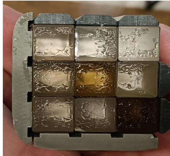
Charge distribution of \text{PbF}_2 pre, after 10 kGy and after 80 kGy irradiation
