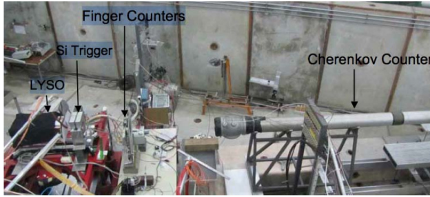
Figure 9.22: Schematic view of the test beam setup used at CERN.
