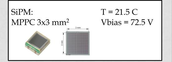
□ Calibration of the gain may be obtained by using the position of the single photon peak in the spectra (corresponding to the amount of charge)
