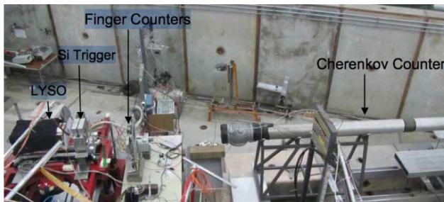
Figure 9.40: Schematic view of the test beam setup used at CERN.
