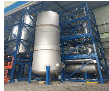
2) Distillation for radiopurity
