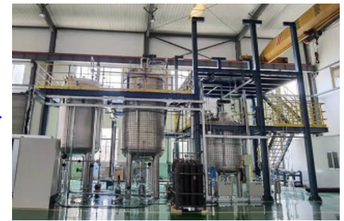
Mixing LAB with PPO and bis-MSB
