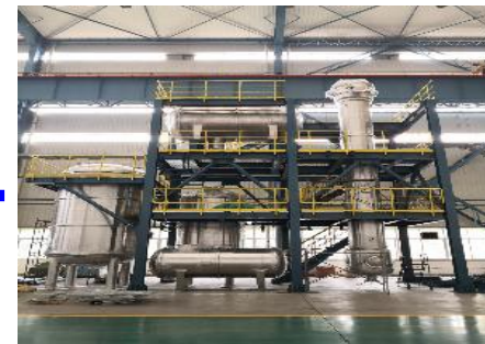
3) Water extraction to remove radioactive impurities
